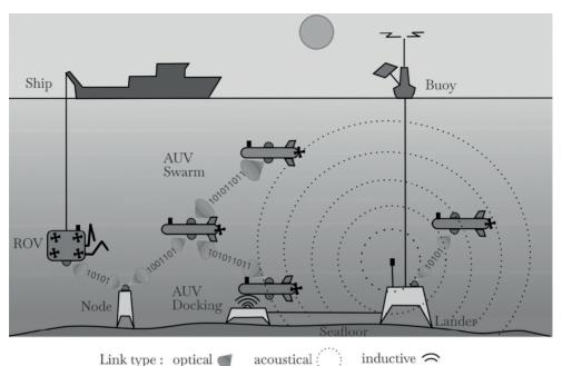
Figure 4 Concept of communication for underwater drone swarming
