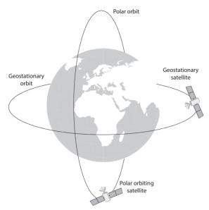
Figure 2 Satellite trajectories (Source: Hardik 2022.)
