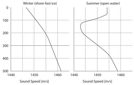
Figure 3 Typical sound velocity profiles in the Arctic, showing the surface channel under the ice in winter and the shallow sound channel at 150m in summer. (Source: Cook et al. 2020, 106.)
