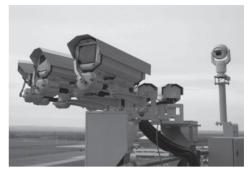
Figure 1 rTWR CWP (left) and rTWR camera configuration (photos taken by the author)
