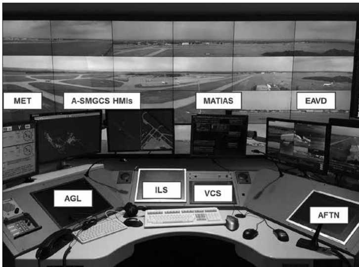
Figure 6. System of Remote Tower Controlling
