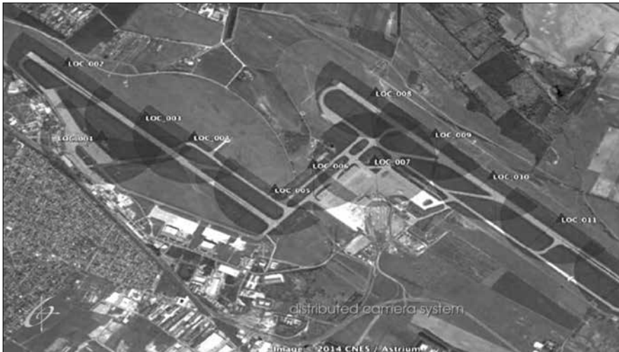
Figure 2. Camera spots' layout at a medium sized airport
