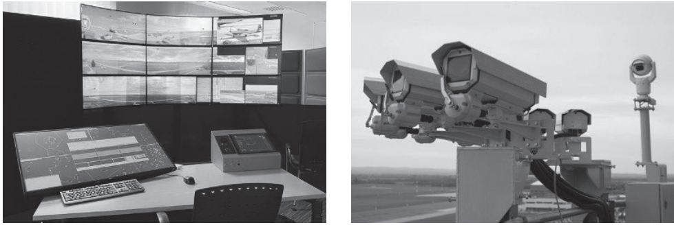
Figure 1 rTWR CWP (left) and rTWR camera configuration (photos taken by the author)
